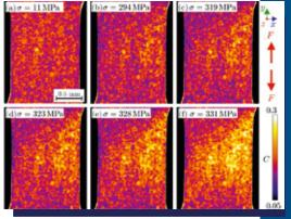
parameters could be achieved in a way unrivalled even by highresolution techniques such as electron microscopy or computed tomography. We present in situ analysis of the damage evolution during tensile load and the identification of void formation in parts produced by selective laser melting.
