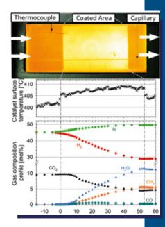
SWIR camera is not influenced by polyatomic molecules partaking in the reactions and thus do not falsify the kinetic data. In this work up to 60 data points per gas species can be collected for 1 experiment. The catalyst mass distribution along the reactor axis is determined using profilometry, enabling the development of a correct model for kinetic parameter estimation and model discrimination. **Guest Speaker**
