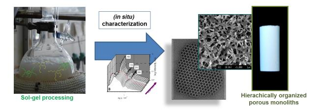
Here, we report on the design of highly porous architectures by sol-gel processing of tailor-made silanes in the presence of structure-directing agents and/or high-internal phase emulsions and post-synthesis treatment of the resulting materials, e.g. by magnesiothermic reduction.
