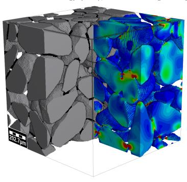
Figure 1: Microstructure and local stress field for a bound sand core microstructure [1]
